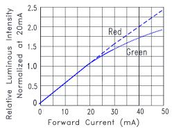
Fig.4 Relative Luminous Intensity vs. Forward Current
