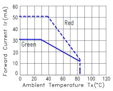
Fig.2 Forward Current Derating Curve
