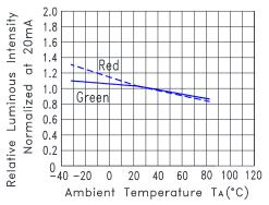
Fig.5 Relative Luminous Intensity VS. Ambient Temperature
