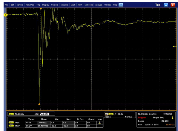
Figure 6. ESD Clamping Voltage Screenshot Negative 8 kV Contact per IEC61000-4-2
