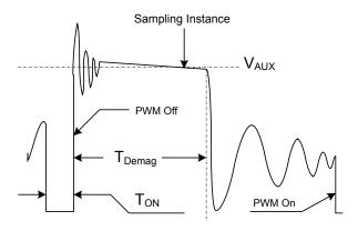
Fig.2. Auxiliary voltage waveform
