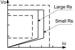
Fig.3 Adjustable output power by changing Rs
