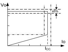
Fig.1. Typical CC/CV Curve
