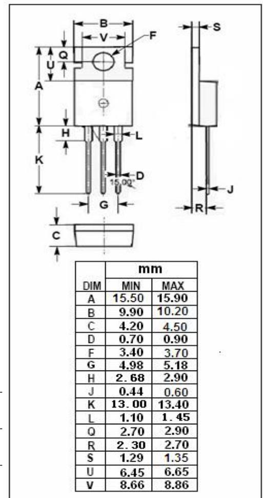
**isc N-Channel MOSFET Transistor**
