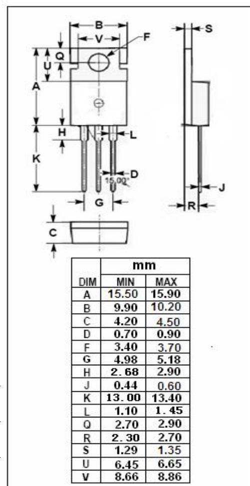
**isc N-Channel MOSFET Transistor****IPP65R280E6, IIPP65R280E6****ELECTRICAL CHARACTERISTICS****T<sub>c</sub>=25°C unless otherwise specified**
