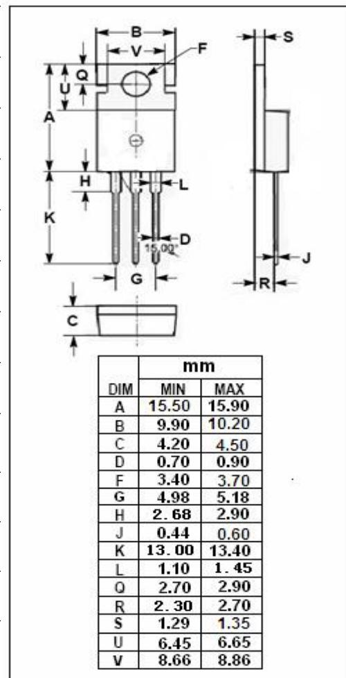
**isc N-Channel MOSFET Transistor****IPP039N04L,IIPP039N04L****ELECTRICAL CHARACTERISTICS****T<sub>c</sub>=25°C unless otherwise specified**
