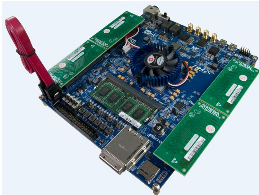
Figure 8-3 SATA Cable and Four FMC Loopback Card Installed
