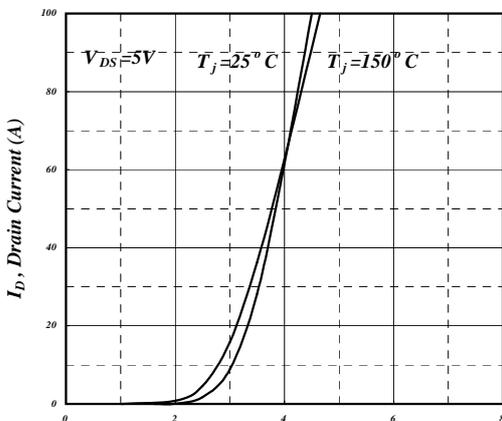
Fig 11. Transfer Characteristics
