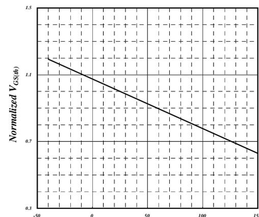
Fig 6. Gate Threshold Voltage v.s. Junction Temperature
