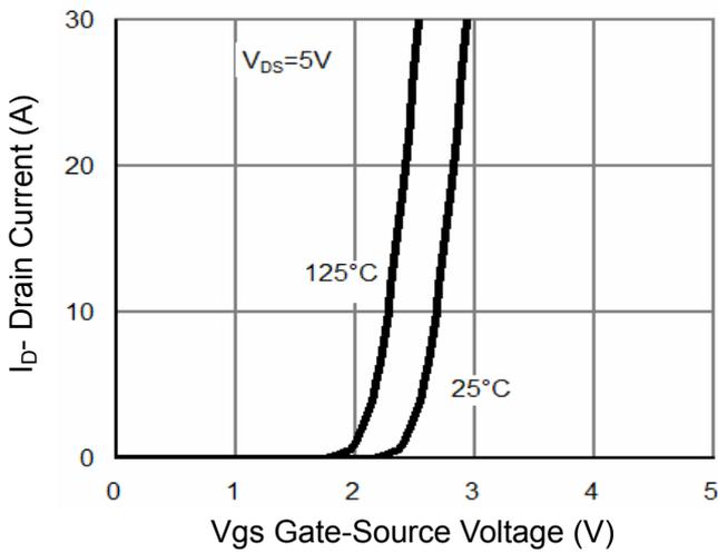
Figure 2 Transfer Characteristics
