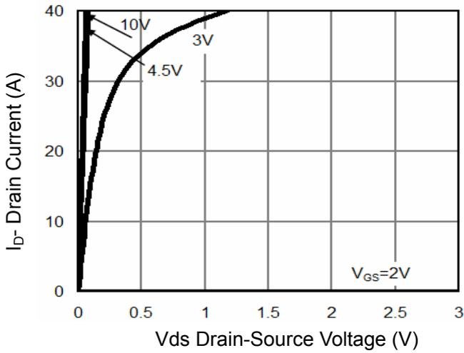
Figure 1 Output Characteristics
