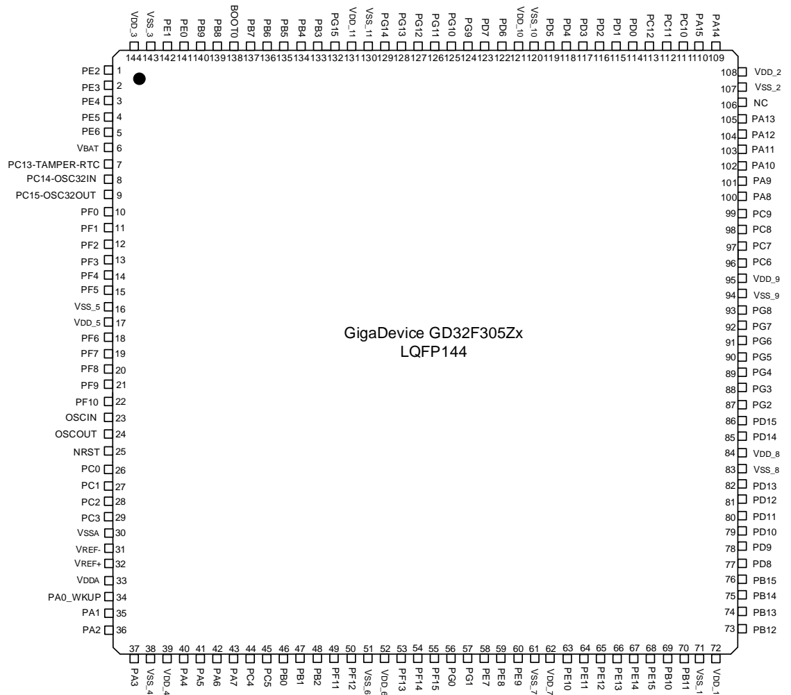
Figure 2-2. GD32F305Zx LQFP144 pinouts
