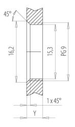
Installation direction: o-ring sits on chamfer.
