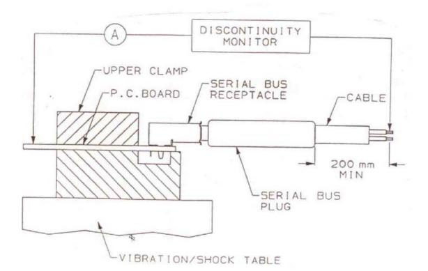
FIGURE 2 VIBRATION AND PHYSICAL SHOCK MOUNTING FIXTURE NUMBER
