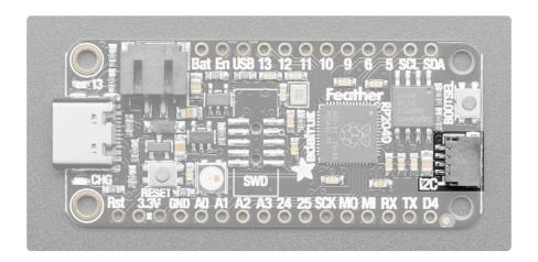
The Feather RP2040 comes with a built in **STEMMA QT connector**! This means you can connect up <u>all sorts of I2C sensors and breakouts</u> (https://adafru.it/18fV), no soldering required! This connector uses the SCL and SDA pins for I2C, which ends up being the RP2040's I2C1 peripheral. In CircuitPython, you can use the STEMMA connector with **board.SCL** and **board.SDA**, or **board.STEMMA\_I2C()**. In Arduino it is **Wire**.
