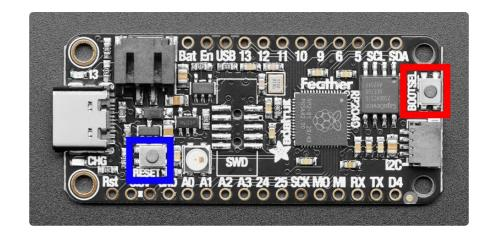
To enter the bootloader, hold down the **BOOT/BOOTSEL button** (highlighted in red above), and while continuing to hold it (don't let go!), press and release the **reset button** (highlighted in red or blue above). **Continue to hold the BOOT/BOOTSEL button until the RPI-RP2 drive appears!**
