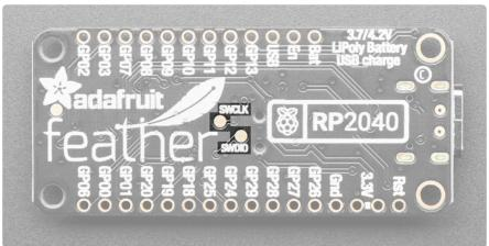
On the back of the board are pads for the **SWCLK** and **SWDIO** pins. They provide access to the internal Serial Wire Debug multi-drop bus, which provides debug access to both processors, and can be used to download code.
