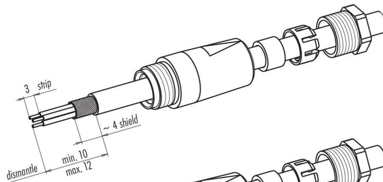
2. Fold shield back, fit collar to cable diameter and solder with shield
