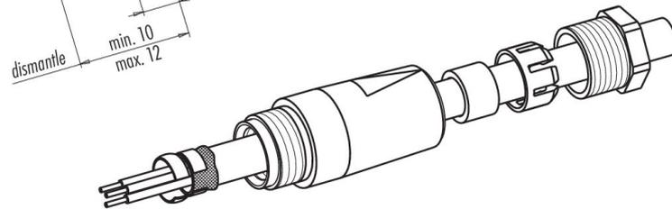
3. Cut off projecting shielding braid, solder insert
