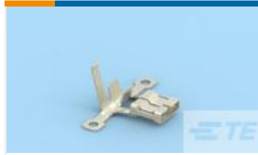
TE Part #2178439-1 250 FASTON, FLAG, REC., 16-12 AWG, PNST
