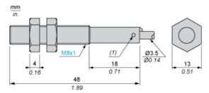
(1) LED, 4 viewing ports at 90° Note Fixing nut tightening torque : <2N.m
