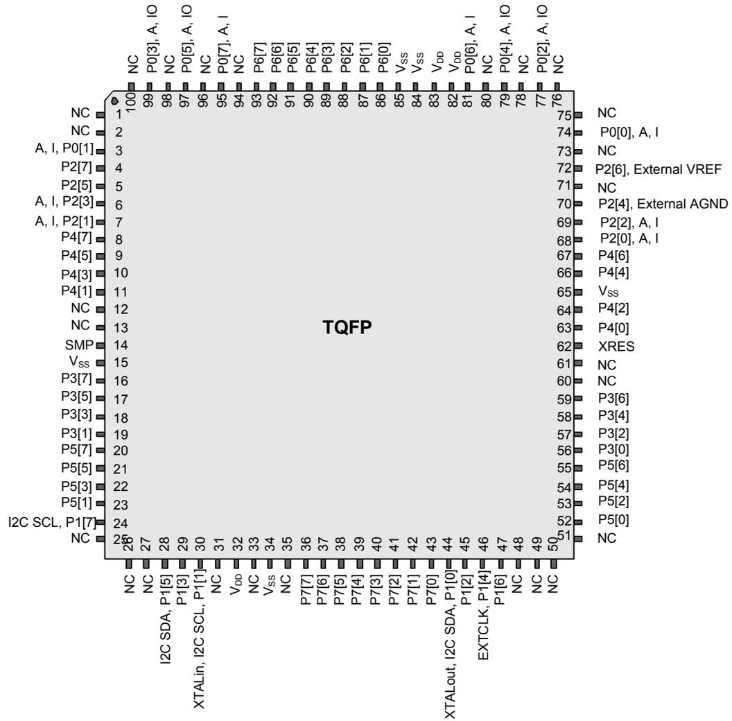
**100-Pin Part Pinout (On-Chip Debug)**
