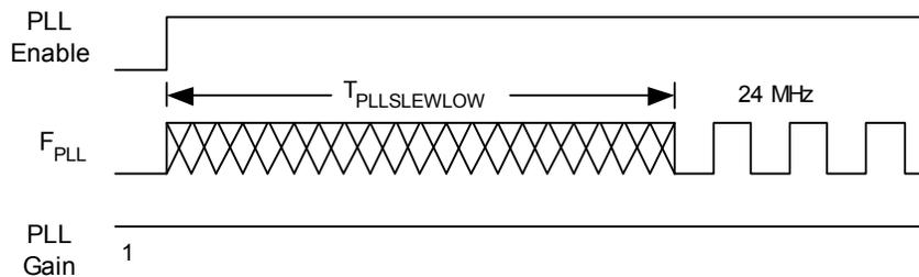
**Figure 14. External Crystal Oscillator Startup Timing Diagram**
