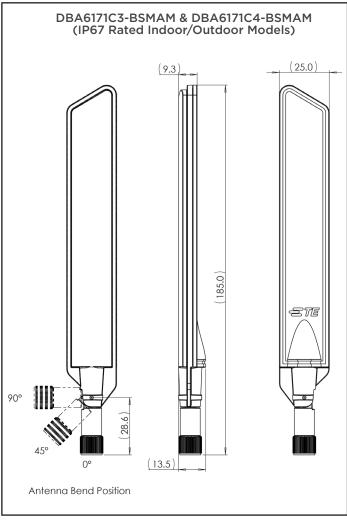
Please note the small difference in connector lengths and overall height between Non-IP and IP67 rated models above.
