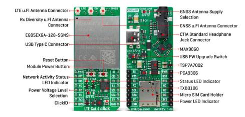
Communication between the EG95EXGA-128-SGNS and the host MCU is made through a UART interface, using standard UART RX and TX pins and hardware flow control pins (CTS/RTS/RI - Clear to Send/Ready to Send/Ring Indicator) for efficient data transfer. The module defaults to a communication speed of 115200bps, allowing for seamless data exchange over <u>AT</u> <u>commands</u>. Notably, this module version also features an audio interface, which can be accessed via the I2C interface.
