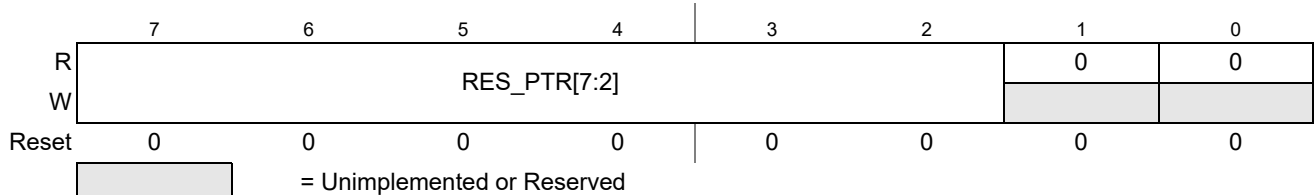
Figure 9-25. ADC Result Base Pointer Registers (ADCRBP_0, ADCRBP_1, ADCRBP_2)
