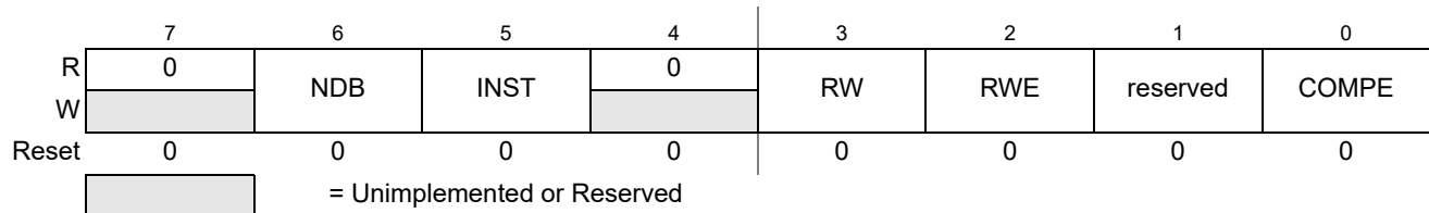
Figure 6-14. Debug Comparator A Control Register
