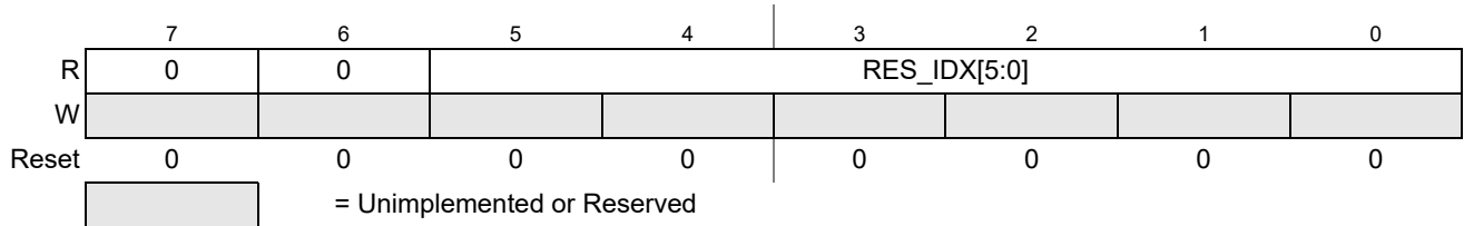
Figure 9-24. ADC Result Index Register (ADCRIDX)
