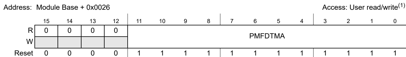
Figure 15-28. PMF Deadtime A Register (PMFDTMA)
