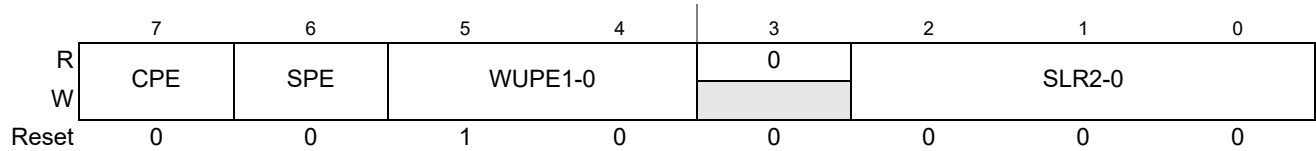
Figure 21-3. CAN Physical Layer Control Register (CPCR)
