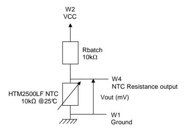
$$V_{OUT}(mV) = \frac{Vcc(mV) * NTC_{HTM2500LF}(\Omega)}{R_{batch}(\Omega) + NTC_{HTM2500LF}(\Omega)}$$
