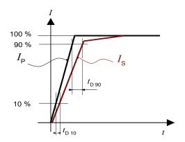
Figure 7:  $t_{D 10}$  (delay time @ 10 %) and  $t_{D 90}$  (delay time @ 90 %)
