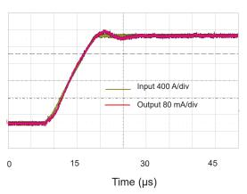
Figure 2: Typical step response (0 to 500 A, 100 A/ $\mu$ s  $R_{\rm M}$  = 1 $\Omega$ )
