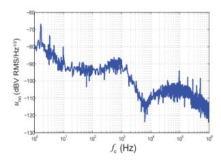
Figure 3: Typical output noise voltage spectral density  $u_{\rm no}$  with  $R_{\rm M}$  = 100  $\Omega$
