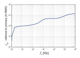
Figure 4: Typical total output RMS noise current with  $R_{\rm M}$  = 100  $\Omega$  (primary referred)
