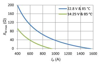
Figure 1: Maximum measuring resistance
