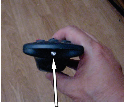
With a button pressed and held, the IR LED doesn't look any different.
