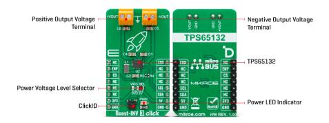
This Click board™ communicates with the host MCU using the standard I2C 2-Wire interface, with a maximum clock frequency in Fast data transfer of up to 400kHz (400kbps). Pulling ENP or ENN pins of the mikroBUS socket to a low logic state turns off either rail (+VOUT or -VOUT, respectively), and pulling both pins to a low logic state turns off the device entirely (the internal oscillator of the TPS65132 continues running to allow access to the I2C interface).
