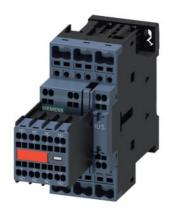
Power contactor, AC-3 25 A, 11 kW / 400 V 2 NO + 2 NC, 110 V AC, 50 Hz 120 V, 60 Hz, with inserted varistor, 3-pole, Size S0 Spring type terminal Captive auxiliary switch
