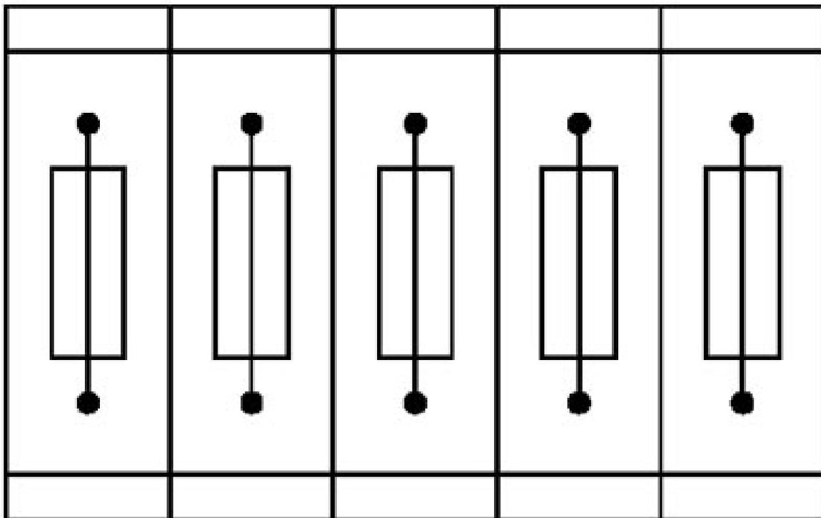
Fuse terminal blocks in interconnected arrangement,
