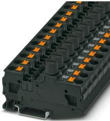
Fuse modular terminal block, fuse type: Glass / ceramics / ..., fuse type: G / 5 x 20, nom. voltage: 250 V, nominal current: 10 A, connection method: Push-in connection, Rated cross section: 6 mm<sup>2</sup>, cross section: 0.5 mm<sup>2</sup>- 10 mm<sup>2</sup>, mounting type: NS 35/7,5, NS 35/15, color: black
