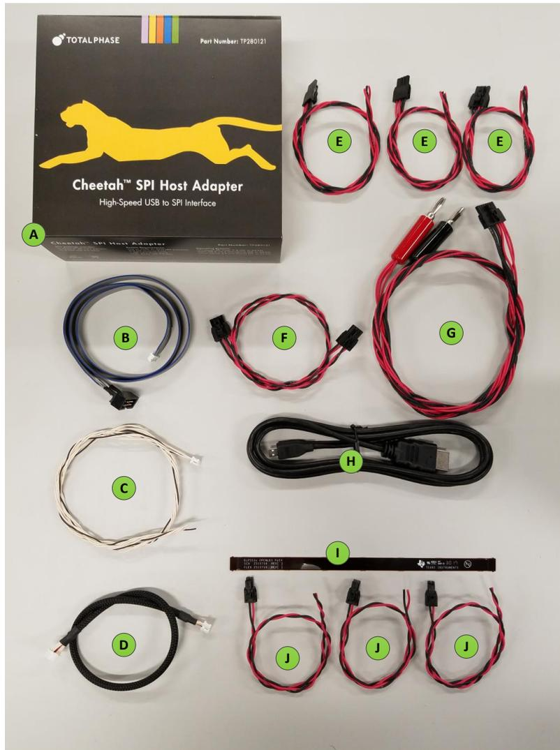
**Figure 3. Cables Included in DLP5531-Q1 Light Engine EVM**
