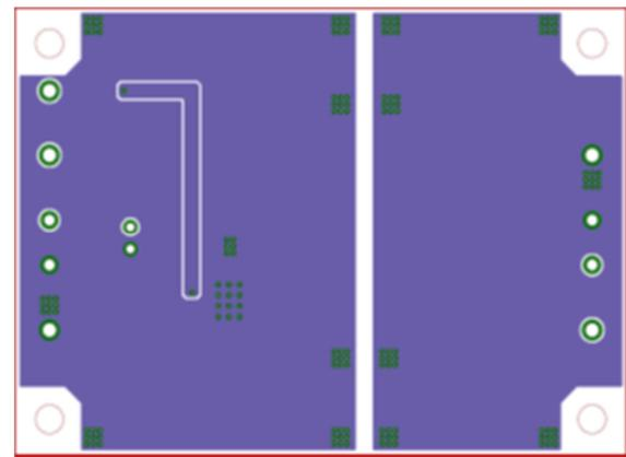
Figure 10. Bottom Side Layer Layout
