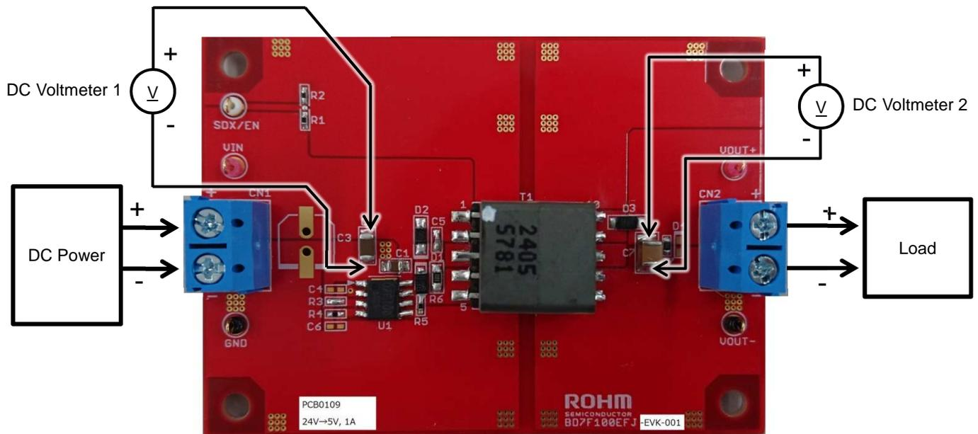
Figure 3. Connection Diagram
