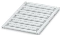
Marker for terminal blocks, can be ordered: by sheet, white, labeled according to customer specifications, mounting type: snap into flat marker groove, for terminal block width: 8.2 mm, lettering field size: 7.4 x 4.7 mm, Number of individual labels: 42
