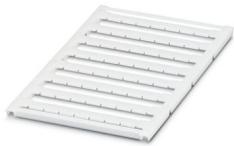
Marker for terminal blocks, Sheet, white, unlabeled, can be labeled with: BLUEMARK ID COLOR, BLUEMARK ID, BLUEMARK CLED, PLOTMARK, CMS-P1-PLOTTER, mounting type: snapped, for terminal block width: 8.2 mm, lettering field size: 7.6 x 5.1 mm, Number of individual labels: 56
