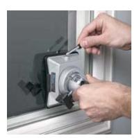
Before you consider a Vacuum Base Repair Kit, clean the pad and then test on a known flat, smooth and nonporous surface like a piece of glass or window.
