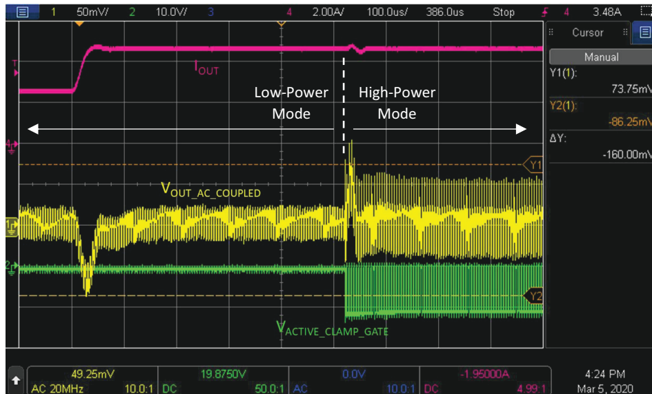
Figure 18. Low-Power Mode to High-Power Mode Transition ( I_{OUT} Changes from 2.6 A to 4.7 A)
