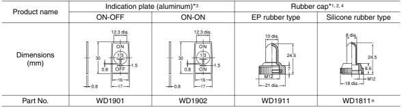
Remarks: 1. The asterisk in the part number WD1811\* for the silicon rubber type rubber cap is where the letter representing the color should be inserted. (B: black; R: red; Z: grey; Y: yellow; G: green.)2. EP rubber cap is available in black only.
