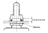
b. Enough screw pitch should be obtained being adjusted within 3 to 3.5mm (See figure above.)
