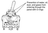
Terminal-sealed type Both switch body and terminals have been sealed to protect from dust and gas that enters from the panel.
