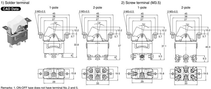
Remarks: 1. ON-OFF type does not have terminal No. 2 and 2. Dimensions of actuator:  $13.4 \times 27$
