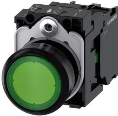
Illuminated pushbutton, 22 mm, round, plastic, green, pushbutton, flat, momentary contact type, with holder, 1 NO, LED module with integrated LED 230 V AC, screw terminal
