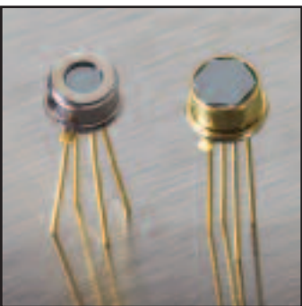
Thermopile Sensors in TO-46 (left) and Isothermal (right) Housing
