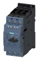
Circuit breaker size S2 for motor protection, CLASS 10 A-release 9.5...14 A N-release 208 A screw terminal Standard switching capacity with transverse auxiliary switches 1 NO+1 NC
