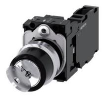
RONIS key-operated switch, 22 mm, round, metal, shiny, lock number SB30, with 2 keys, 2 switch positions O-I, latching, actuating angle 90°, 10:30h/13:30h, key removal O+I, with holder, 1 NO+1 NC, screw terminal, possible special locks: SB31, 421, 455 lower case
