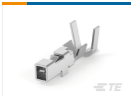
TE Part #1827587-2 Contact: Component To Wire; 3-5A, 30-18 Wire Size
