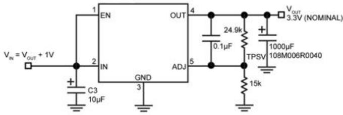
Figure 2. IFX1963 Load Transient Response Test Circuit
