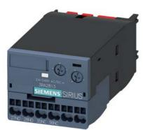
solid-state time-delayed auxiliary switch, ON-delay, relay 1 NC + 1 NO, time range 0.05-100 s, 24-240 V AC/DC, 50/60 Hz, varistor for attenuation of the contactor coils integrated, spring-loaded terminal, can be snapped onto the front on contactors 3RT20 and contactor relays 3RH2
