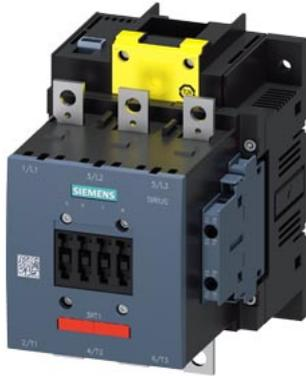
Power contactor, AC-3 185 A, 90 kW / 400 V Coil AC 50/60 Hz and DC 96-127 V x (0.8-1.1) F-SPS input 24 V DC 3-pole size S6 Auxiliary contacts 2 NO + 2 NC permanently mounted Main circuit: Busbar Control and auxiliary circuit: Screw terminal
