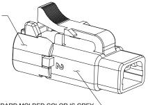
2 POS, PLUG, SOCKET, ATM SERIES, SNAP FIT
