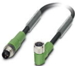
Sensor/actuator cable, 3-position, PUR halogen-free, black-gray RAL 7021, Plug straight M8, on Socket angled M8, cable length: 2 m
