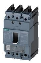
circuit breaker 3VA5 UL frame 125 breaking capacity class S 25kA @ 480V 3-pole, line protection TM230, FTAM, In=60A overload protection Ir=60A fixed short-circuit protection Ii=5...10 x In without connection
