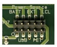
Depending on the power source, make sure you connect jumpers to the appropriate pins on the "Power Source" header. For instance, if you use batteries, use a jumper to short-circuit pin 1 and 2 on the header. The last jumper in the row (pin 9-10) should always be mounted, unless the MSP430 FET is used as the power source.
