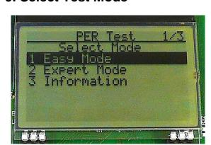
The PER test can be run is several modes. Easy Mode sets up a one-way test and uses default settings. This test is convenient for practical range testing.
