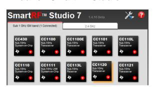
After installing the tool, connect the EB to the PC using the USB cable and start SmartRF Studio. Select the "Sub 1 GHz" tab and double click the highlighted CC1120 or CC1121 device icon.
