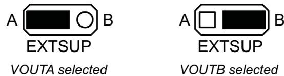
**Figure 7. EXTSUP Jumper Setting**
