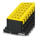
High-current terminal block, nom. voltage: 1000 V, nominal current: 145 A, number of connections: 2, number of positions: 1, connection method: Screw connection, Rated cross section: 50 mm<sup>2</sup>, cross section: 6 mm<sup>2</sup> - 50 mm<sup>2</sup>, Rated cross section: 50 mm<sup>2</sup>, cross section: 4 mm<sup>2</sup> - 50 mm<sup>2</sup>, mounting type: NS 35/15, NS 35/7,5, color: yellow
