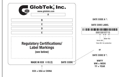
A=ICT / ITE / Medical Power Supply B=P/N: (料号) WR9HA2000LCPMFR6B C=Model (型号) GTM86100-1005-W2 D=Input (输入)100-240V~, 50-60Hz, 0.3A E=Output (输出)5.0 V == 2.0 A, 10.00W
