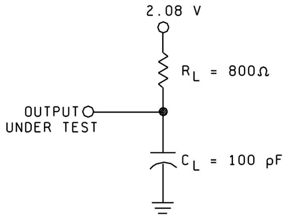
FIGURE 4. Output load circuit.
