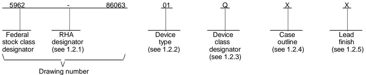
1.2.1 RHA designator. Device classes Q and V RHA marked devices meet the MIL-PRF-38535 specified RHA levels and are marked with the appropriate RHA designator. Device class M RHA marked devices meet the MIL-PRF-38535, appendix A specified RHA levels and are marked with the appropriate RHA designator. A dash (-) indicates a non-RHA device.
