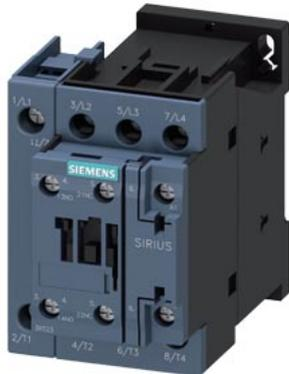
contactor AC-1, 35 A, 400 V / 40 °C, 4-pole, 24 V AC, 50 Hz, auxiliary contacts: 1 NO + 1 NC, screw terminal, size: S0
