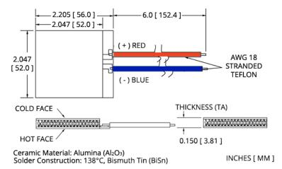
Ceramic material 96% Alumina ceramics Solder construction: 138°C BiSn
